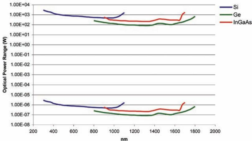
\*The above graph indicates the maximum power that can be introduced in the sphere before detector saturation appears. The maximum useable power range for Labsphere's LPMS systems is determined by the thermal stability limits of the sphere coating/material, which should not exceed 400°C for Spectralon, 100°C for Spectrafect, and 500°C for Infragold.
